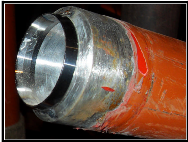
Machine Beveled Insert (Fit and Tacked)
